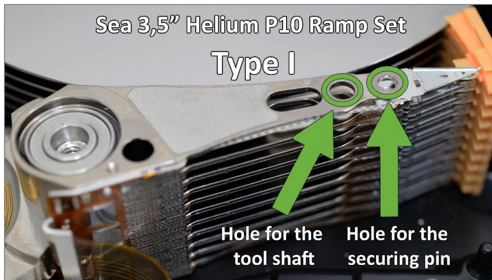
(Picture 1: HSA with holes for the tool shaft and securing pin – Sea 3.5" Helium P10 Type I tool)
