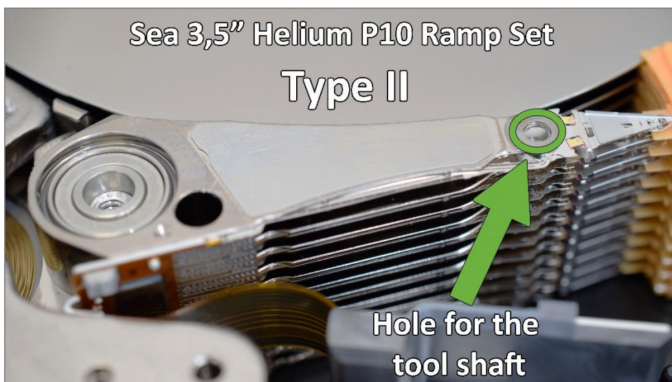
(Picture 2: HSA with only a hole for the tool shaft – Sea 3.5" Helium P10 Type II tool)
